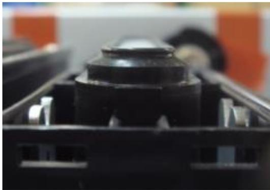
Wrong position: The snap-fit is not engaged.
