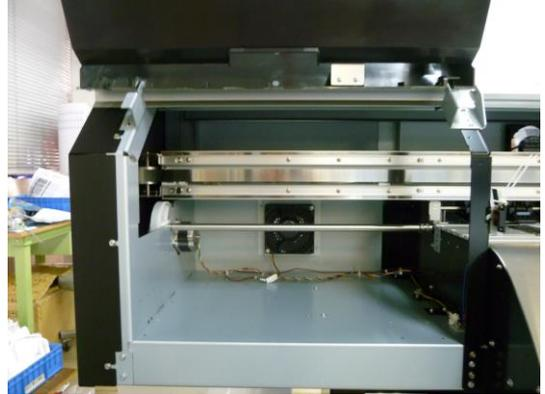
2. Remove the two screws securing the FAN(REAR)ASSY MW, disconnect the connector, and then remove the FAN(REAR)ASSY MW.
