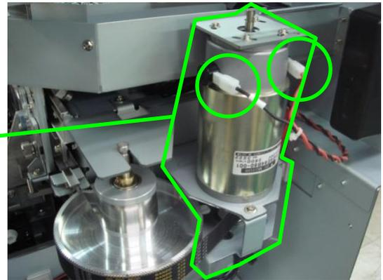
5. Remove the BRACKET(Y-MOTOR-SUPPORT) and the BRACKET(DSE64B-MAIN)-MW with five fixing screws, and then remove the Y-DRIVE-MOTOR-ASSY and the DRIVING PULLEY together.
