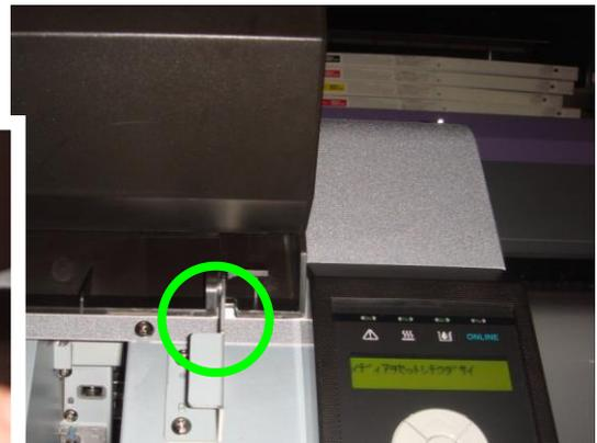
With the COVER(R)ASSY-MW open, push the lever on the top right upward as shown in the picture, and while keeping the pressure move the COVER(R)ASSY-MW to the left.
