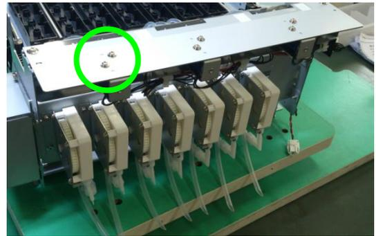
3. Disconnect the SOLENOID ASSY(MV) connector, and remove the SOLENOID ASSY(MV).
