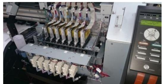
5. Check the linear encoder horizontal position in both home and maintenance area positions. Adjust the horizontal position if not correct.
