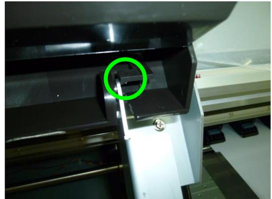
4. Slide the COVER(L)ASSY-MW (or COVER(R)ASSY-MW) to the left, remove the right and left hinges, and remove the cover.
