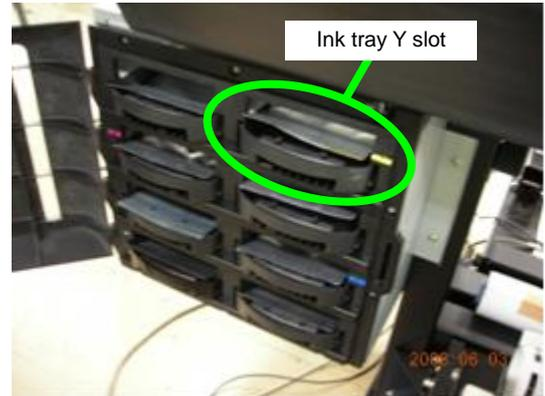
3. Place your hand inside the ink tray Y slot, grab the PHOTO SENSOR 5 (cover sensor) tab, and remove it by pulling it in the upward direction.
