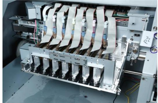
2. Loosen the two screws securing the REGISTRATION-ENCODER, and adjust the position by moving the REGISTRATION-ENCODER up and down. Adjust the linear encoder position so that the T fence upper edge matches the linear encoder corner.
