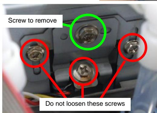
6. Remove the two screws securing the LINEAR ENCODER ASSY(MW). Then cut the insulok cable tie fixed to the BRACKET-ENCODER-S, and remove the LINEAR ENCODER ASSY(MW).
